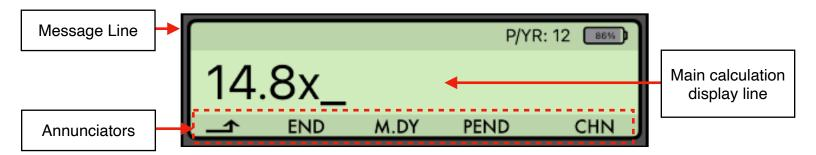
The RLM-14B calculator's display has three areas: the message line, the main calculation line and the annunciators line.
