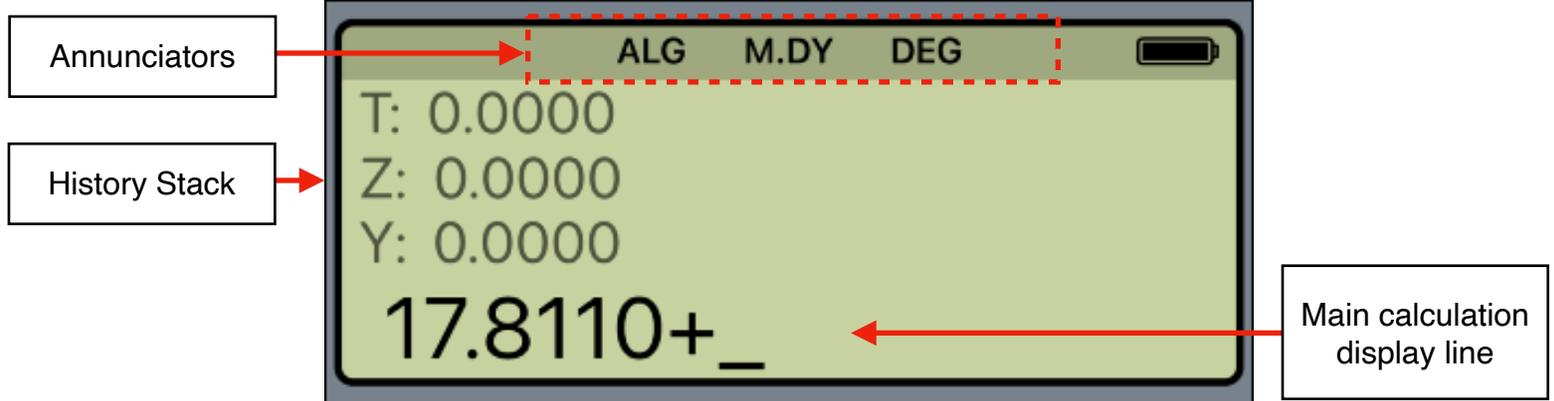
The RLM-17BX calculator’s display has three areas: the annunciators area, the history stack area and the main calculation.
