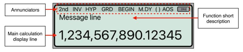
The RLM-BA" calculator's display has three areas: the message line, the main calculation line and the annunciators line.
